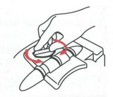
The best adjustment may allow you to see only three marks, or four slightly blurred marks. When you have completed the IPD adjustment, proceed with the FOCUS adjustment.
