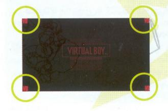
The best adjustment may allow you to see only three marks or four slightly blurred marks. When you have completed the IPD adjustment, proceed with the FOCUS adjustment.
