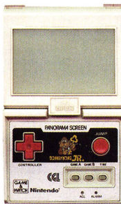
Yokoi's Game & Watch handhelds pioneered the use of the now familiar d-pad controller
